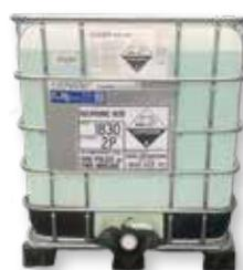
Sulphuric acid is commonly used to regenerate strong acid cation resins associated with Ion Exchange Systems.
